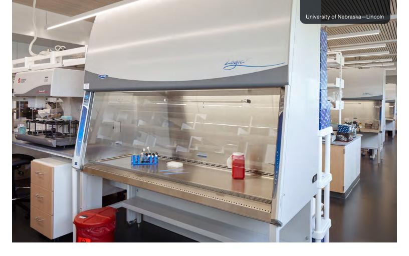
three main divisions: Type A, B and C. Class II, Type A BSCs recirculate air back into the lab. Unless however, they are canopy connected to the outside as required by the application (work with odorous materials). Class II, Type A1 and A2 BSCs are similar, yet separated by the minimum average inward air velocity required. Type A BSCs cannot handle work involving radionuclides or hazardous chemistry.
