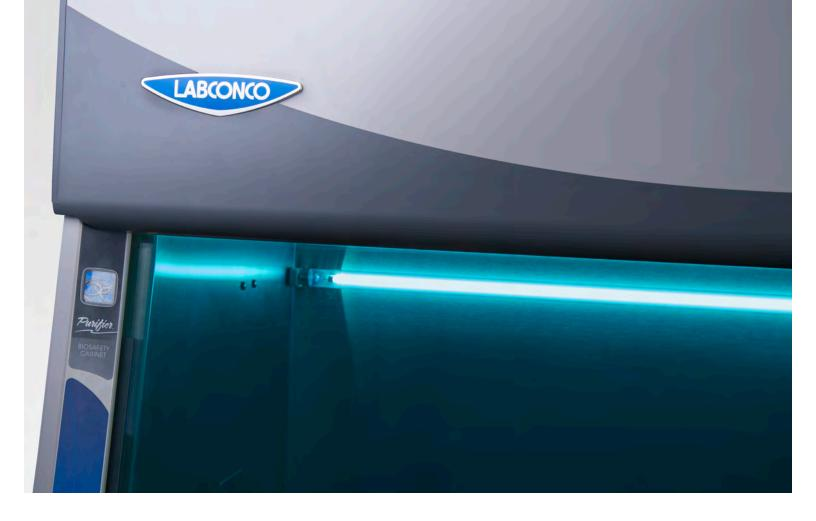
that for UV lamps to be effective, the target **must** be in direct line of sight with the light source. This is bad if you are using a germicidal lamp as the primary decontaminant in your lab's culture enclosure.
