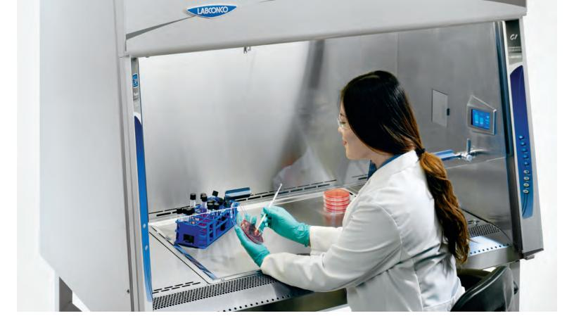
Airflow requirements closer to an A. The large volume of air needed to exhaust a B2 BSC is a leading cause of initial lab commissioning failures. Why? Modular cleanrooms are limited in their overall size, and B2 BSCs require more than many air handling systems and rooms can provide.
